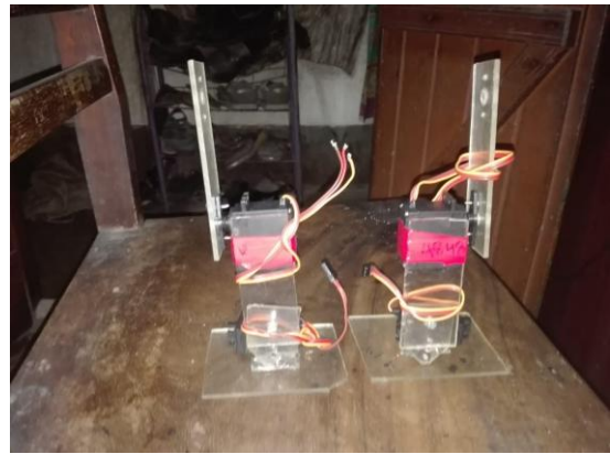
Fig 3: Initial Leg Design with Perspex Plastic.
