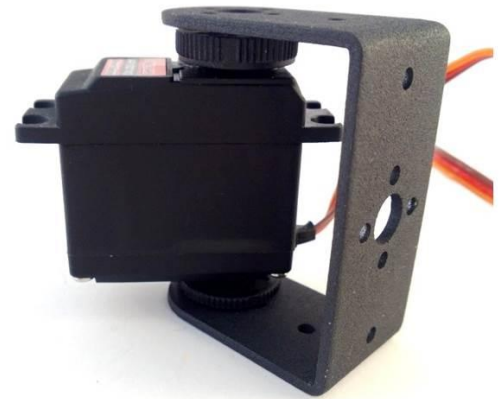
Fig 4: Actuator Joint with aluminium bracket .
